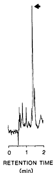
Figure 4. Chromatogram of a \text{CO}_2 supercritical fluid extract of whole meal flour obtained from a commercial bakery. Injection of 20 \mu\text{L} was equivalent to 100 \text{ mg} of flour. Analysis was performed with supercritical \text{CO}_2 containing 10% methanol at 50^\circ\text{C} and a pressure of 302 bar on a 250 \times 4.6 \text{ mm} i.d. stainless steel column of Spherisorb Amino 3 \mu\text{m} . Ultraviolet detection was at 282 nm.
